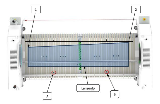
The error A50 shows that the bed sheet in progress on the first crossfold table has the ends (1) and (2) not in line. This check is done by the photosensors (A) and (B)
