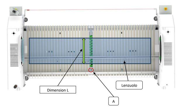
The errore A49 shows that the bed sheet in progress on the first crossfold table has the dimension L greater than the maximum allowed dimensions to be folded. This is a safety check to avoid line jam.
