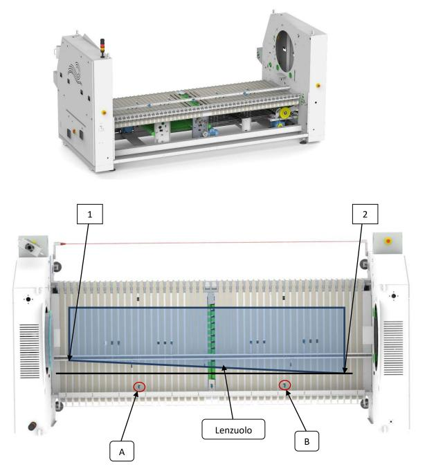
The error A51 shows that the bed sheet in progress on the first crossfold table has the ends (1) and (2) not in line. This check is done by the photosensors (A) and (B)
