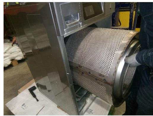
**Step 8:** Insert the drum shaft with tightening until it stops so the shaft and bearings are aligned. Use a hydraulic pump or similar for it.
