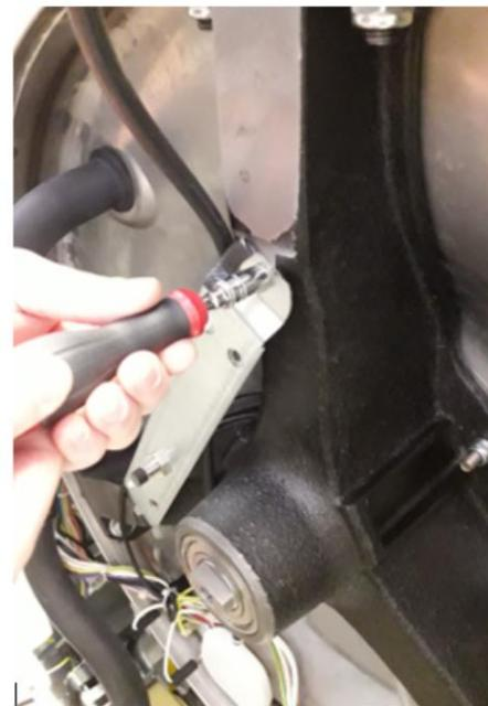
**Step 2:** Move the overflow pipe and the pressostat to one side in order to remove the bearing support.
