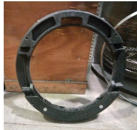
**Step 5:** Remove the counterweight and the front of the tub.
