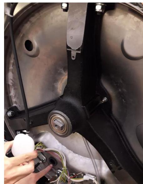
**Step 3:** Undo the three bearing support bolts and the six bolts on the crosspiece.
