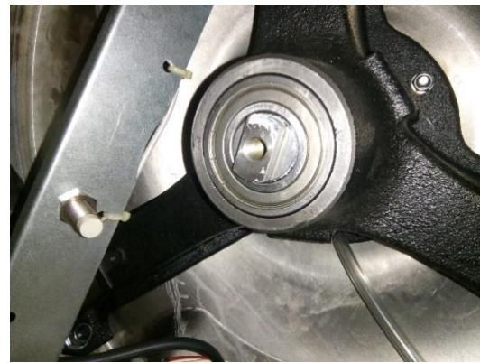
**Step 9:** Replace the pulley, sensor support and the panels.
