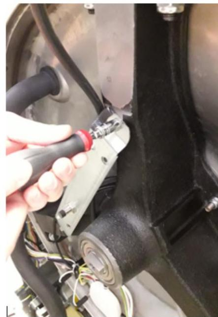
**Step 3:** Remove the door, the door base and the lock. It is not necessary to release the lock completely, just releasing the two screws as it is shown in the image and moving it to the side is enough.
