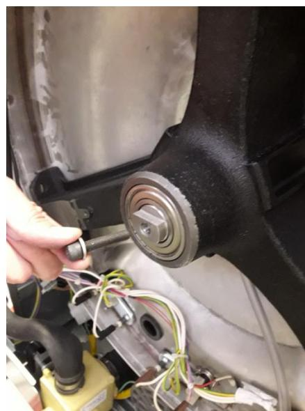
**Step 5:** Remove the bearing support using the extractor.
