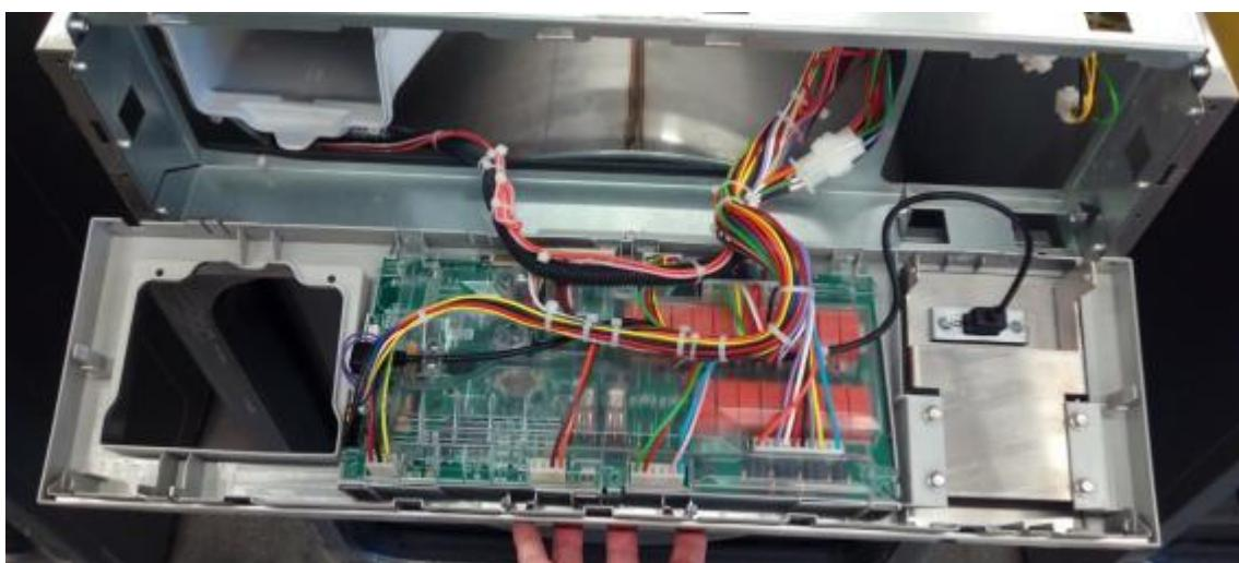
**Step 9:** Release the USB connector (A) and lower flanges (B) of the cover.
