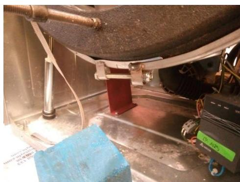
**Step 10:** Tighten the pulley screw and the screws of the motion sensor to fix them.
