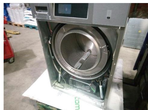
**Step 6:** Release the drum with the help of an extractor. It is important to place a screw to support the extractor without damaging the thread.
