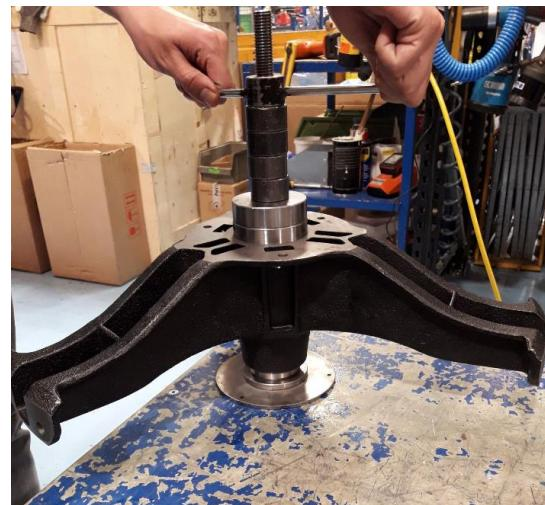
**Step 8:** Insert the drum shaft, tightening it to the limit so that the shaft and the bearings are correctly aligned. Use a hydraulic pump or similar for this operation.
