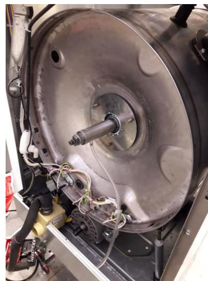
**Step 6:** Remove the bearings from the support.
