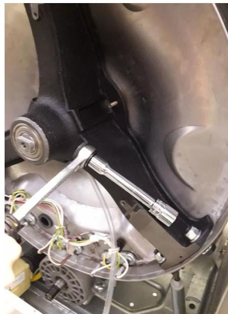
**Step 4:** Insert a safety bolt to protect the thread of the shaft.
